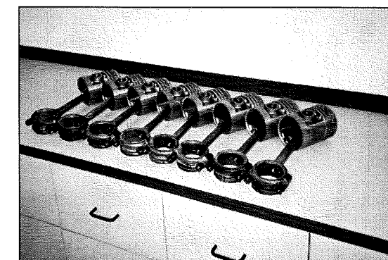
The eight piston and steel connecting rod assemblies from the Duesy engine just prior to restoration showing large chunks of missing bearing babbitt—a major event in the making.
