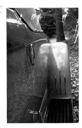
Massive door hinges along with running board and fender details
