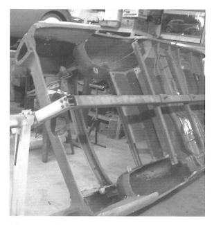
*Photo #3: The 1953 Mercury body has had the* rear cross bar loosened and moved forward out of the way to permit total removal of a rustedout trunk floor. The body has been prepared for installation of the replacement floor-board section. *The body is adequately supported to do this major* repair by just four ½-inch all-thread attachments.
