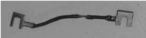
What to look for -- worn out insulation on the wire.
