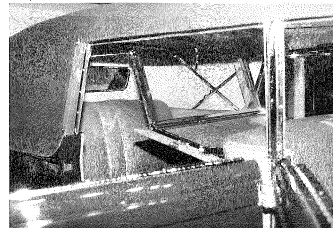
Unique folding rear windshield in the Duesenberg.
