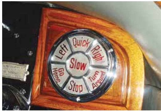
Panel Providing Instructions to Chauffeur Controlled in Passenger Compartment
