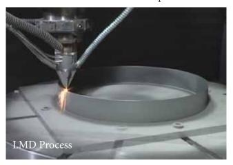
**2. Direct Energy Deposition (DED or LMD):** This process works like the plastic 3D printer. A narrow rod of powdered metal (like a welding rod) moves very slowly down toward the printing base, and a highly controlled
