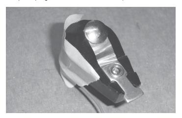
Step 6: Tape or hot-glue a fine, non-stranded wire onto the rotor as pictured. The location of the wire doesn't matter; only that it be a small diameter and be securely fastened so it doesn't move. The end must sit just above the top edge of the distributor body.
