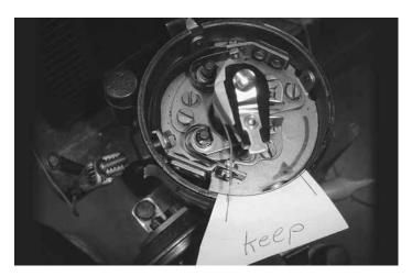
**Step 9:** Remove plastic insulator, and slowly rotate distributor shaft. If both points-sets are correctly synchronized, the light will come on, and then go out as the pointer crosses the left-hand line on the paper segment. If the light goes out (points open) before or after the wire meets the left-hand line, move the base (not gap) of the moveable points (right points in photo) until the light goes out when the wire crosses the line.
