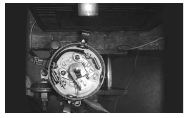
**Step 7:** Attach a test light between the coil terminal on the distributor body and a battery. (Car battery, flashlight battery; doesn't matter. Use appropriate bulb). Place a ground wire from the other battery terminal to the distributor body. As you rotate the distributor shaft, the light will go on when either points are closed, and off when both points are open.
