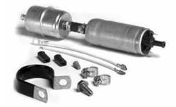
number is P60430. This pump is not recommended for priming the carburetor or other intermittent use. The reason is that the gear/rotor mechanism restricts fuel flow when the pump is not running, and if the gear and rotor end up in just the right (actually, wrong) position when the pump is switched off, the pump can block fuel flow completely.
