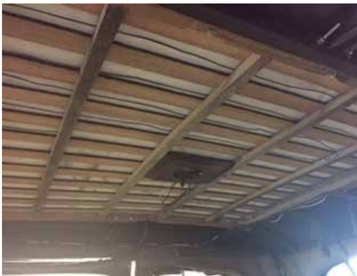
The completed top bows for the roof of the Cadillac V16 Sedan
