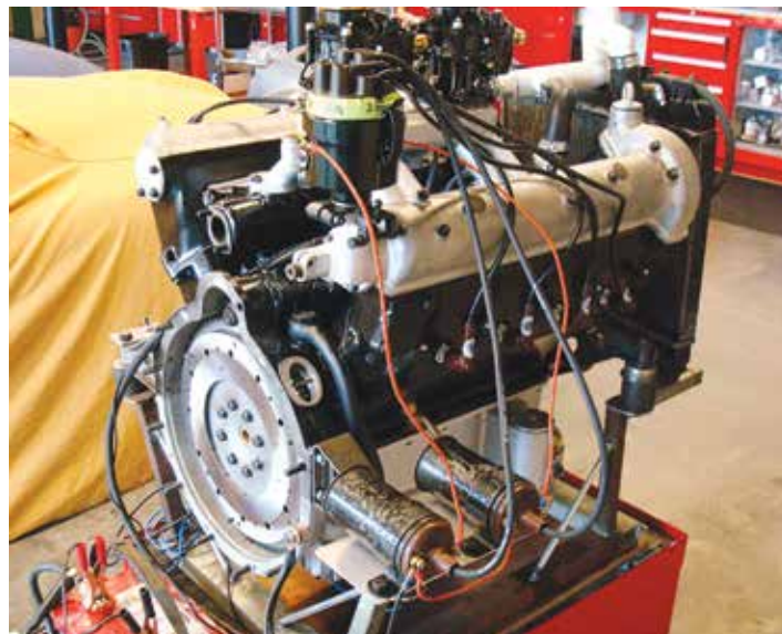
"The near complete S11 engine being test run."
