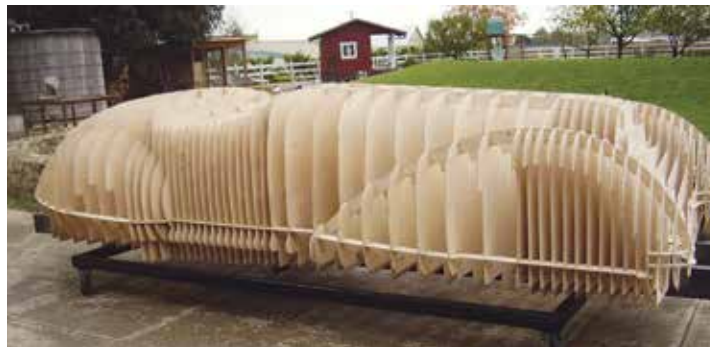
The body buck consists of slices used to fit the aluminum panels
