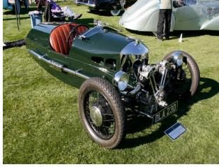
Brian started at 10-year restoration project on it in 2002. The engine was overhauled with many new bits including pistons, bearings, and oil pump. The body wood structure was rebuilt with new ash members where required and the sheet metal was replaced as needed.
